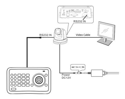
The RMC-190 PTZ Camera Control Unit can also be used in an environment where multiple cameras are required. With RS-232 INPUT/OUTPUT ports, the user is allowed to control up to seven cameras connected in a daisy chain fashion.
