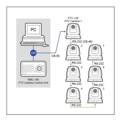
However, it should be noted that the connection will be broken if one unit is powered off. In other words, the cameras connected subsequent to the broken one will become uncontrollable by RMC-190. For example, in the above diagram, if cameras #2 and #3 are defective or powered off, all camera connections (4/5/6/7) after camera #3 will be cut off from the daisy chain and RMC-190 will not be able to control them even if the cameras are still operable.
