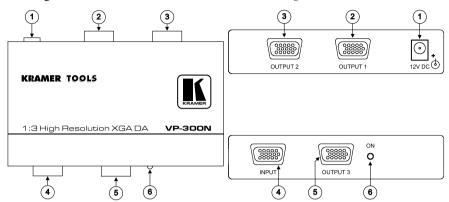
Figure 2: VP-300N 1:3 High Resolution XGA DA
