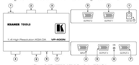
Figure 3: VP-400N 1:4 High Resolution XGA DA
