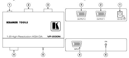
Figure 1: VP-200N 1:2 High Resolution XGA DA
