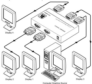
Figure 5: Connecting the VP-400N to 4 Displays
