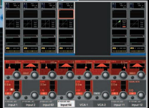
User configurable layers place channels and outputs within easy reach of the operator.
