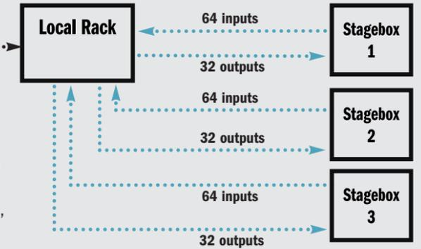
Vi consoles support up to 5 stageboxes. This means that a digital patchbay can be created, where the engineer can select the 64/96 inputs to a Vi6/Vi2 (or 48/72 on a Vi4) from a selection of inputs available on any of the connected stageboxes. So, for example, with two stageboxes connected there are 128 inputs to select from, with three there would be 172, and so on, up to a limit of 192 channels, which is the combined maximum of local plus stagebox inputs.
