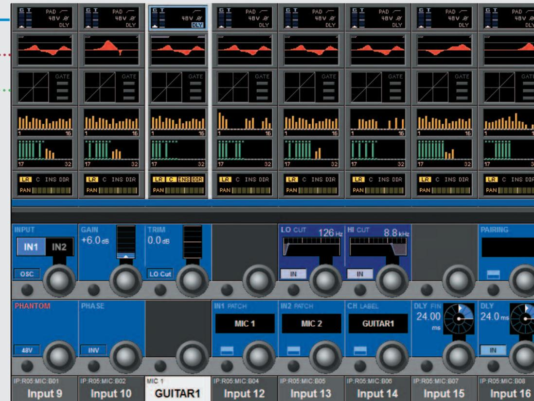
The 16 switches and rotary encoders change function according to the mode selected. This real 'where you look is where you control' philosophy makes operation of a Soundcraft Vi Series™ console highly intuitive.
