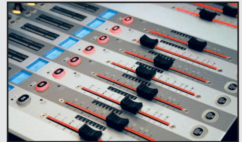
Bringing up the output channel strip and touching the Graphic EQ button immediately assigns the first 30 faders on the console to Graphic EQ, with the Soundcraft FaderGlow™ changing to red, indicating that the console is no longer in channel fader mode.
