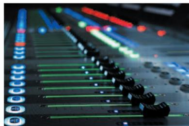
Assignable faders are an inevitable part of digital mixing. But assignability can quickly lead to confusion. That's why we developed Soundcraft FaderGlow™ for the Soundcraft Vi Series™ – a clever yet simple idea to illuminate the fader track in colours that integrate with those of Vistonics™ II to show, at a glance, what function a fader is controlling at any given time.
