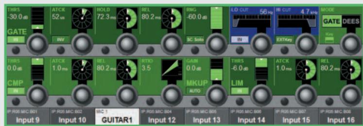
The dynamics section controls a Noise Gate with attack, hold and release, and a key facility with filtering. The Gate can be replaced with a De-Esser function. Working in series with the Gate, the full-function Compressor maps gain reduction metering onto the LED meter in the fader area, with full control of threshold, ratio and release with an independent Limiter section and overall gain makeup.
