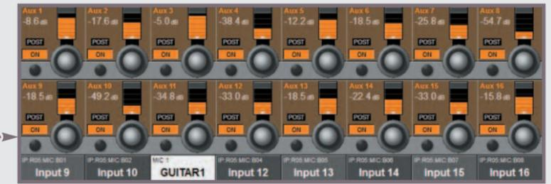
Two areas of the channel strip allow access to routing and control of the output busses, arranged in two banks. The ALL BUSSES mode allows assignment of each of the busses as an Aux, Group, or Matrix output (maximum of 16 Matrix busses possible), with additional stereo pairing controls if busses are required as stereo sends.
