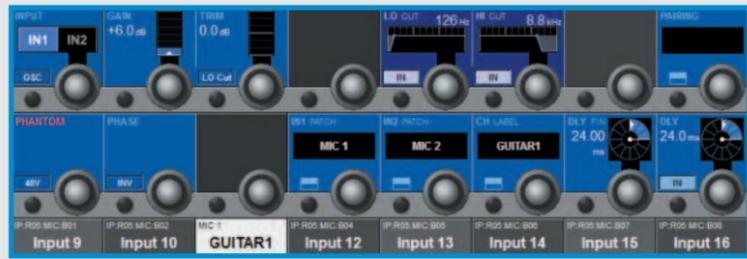
The blue input stage and routing screen allows adjustment of input delay, mic gain, digital trim, high and low-pass filter frequency, channel patching, channel naming and stereo pairing.
