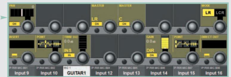
The final section of the channel strip controls the Pan, Insert and Direct out functions, with assignable LR and C, or LCR panning modes. Inserts can be switched pre or post EQ/dynamics, with the Direct output send assignable to pre-filters, pre-EQ/dynamics, post EQ/dynamics and post-fade points.
