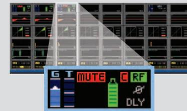
Shows the wireless mic status directly on the relevant channel strip. VM<sup>2</sup> displays battery life, RF status and mute status.
