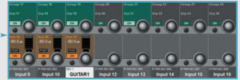
Subsequently within each channel strip setup, busses can be switched on or off with level control, or switched pre or post fader, with a global mode allowing pre or post EQ/dynamics.
