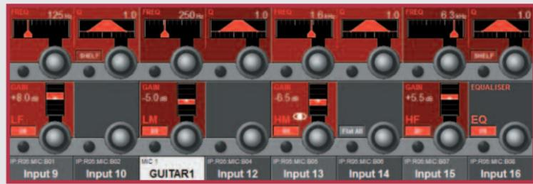
The four-band fully parametric EQ is graphically displayed with the settings for boost/cut, frequency and Q (bandwidth), with the main screen showing the composite EQ curve. Frequency is displayed in a similar style to a radio tuner scale for easy assimilation, and the HF and LF bands can be switched to shelving EQ.
