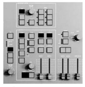
These controls set the general operating conditions for the entire desk. The Master functions determine the mode of operation, the functions of the buttons throughout the desk, and the maximum output level for any channel.
