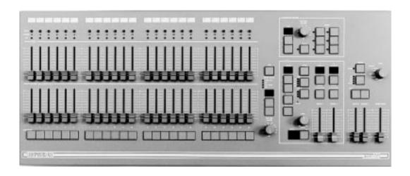
The memories in the Lightmaster XLS are arranged in 9 pages, each of 24 memories. The B Preset Faders become 24 Memory Masters In Run and Program Mode. This provides an easy way of recording up to 216 scenes which would otherwise have to be set up manually on the Presets. Any scene may be previewed (indicated on the Preview lights), before it is output.
